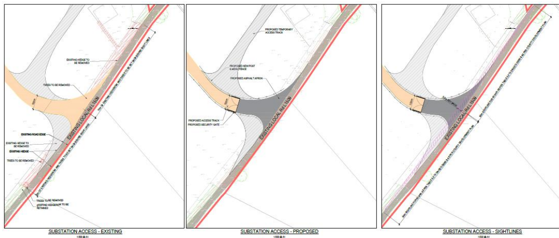
FIGURE 2.3: SUBSTATION ACCESS ASSESSMENT EXTRACT
